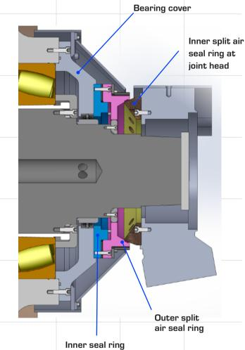
The new split design eliminates the need to disassemble the joint head to remove the seal, allowing easy replacement. The seal air gap can also easily be adjusted by adding shims. The result is improved sealing performance and increased operational reliability.
